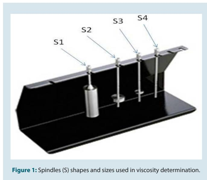
Figure 1: Spindles (S) shapes and sizes used in viscosity determination.
