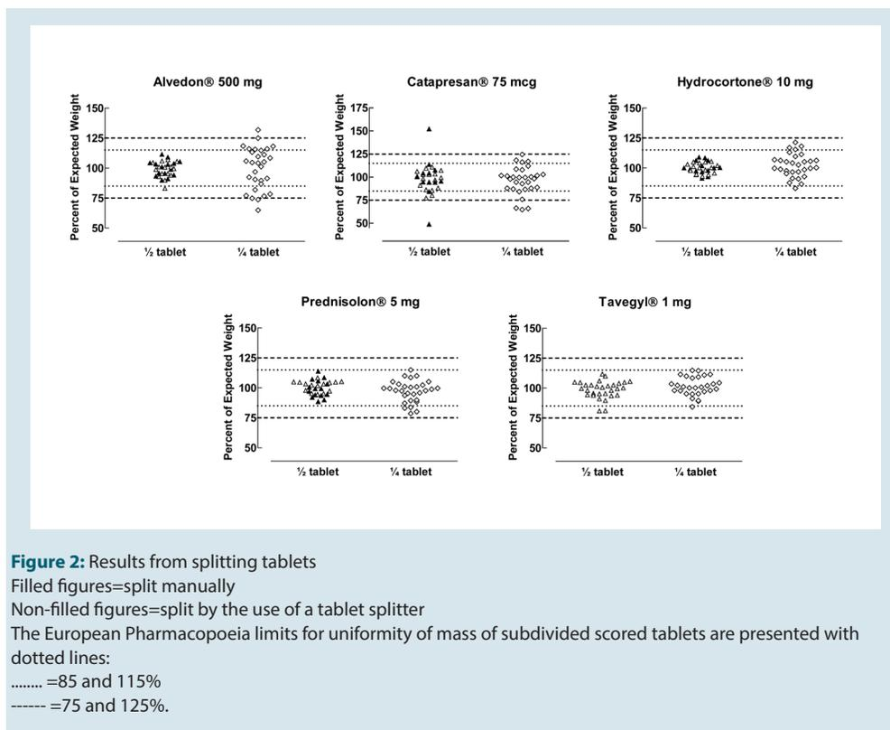
to paediatric patients. The tablets chosen also represent a wide variety of sizes. To avoid inter-individual variability the data presented in this report are the results of one paediatric pharmacist (ÅÅ) splitting the tablets using a tablet splitter in the pharmacy and using a pair of thumb forceps when lifting the halves or quarters onto the scale.
