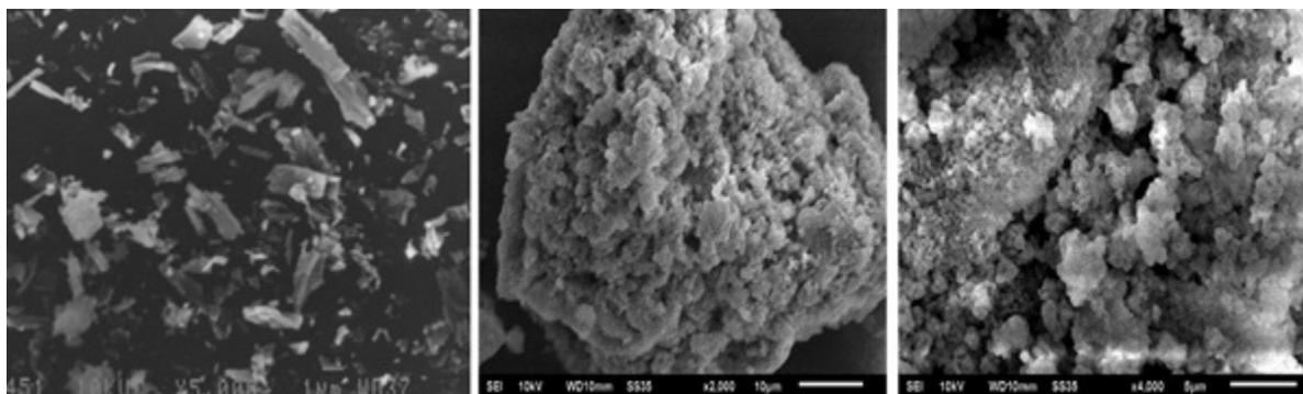
Figure 4: SEM of a) Pure ATV b) S-SMEDDS (SF2) c) Neusilin US2
